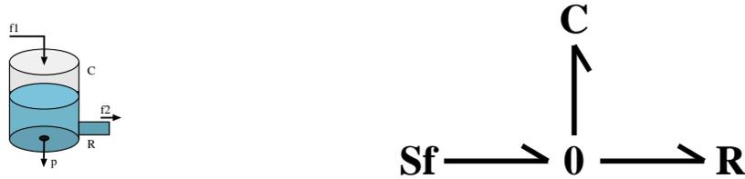
Figure 2: One-tank fluid system and bond graph.
