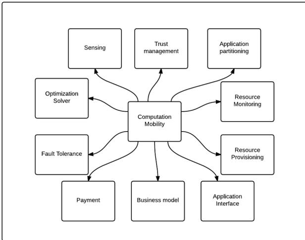
Fig. 1. Components of a Computation Mobility Framework
