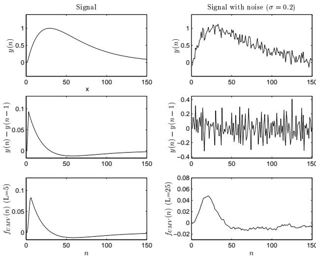
Fig. 3. Comparison of derivative estimation with a first-order difference operator, and an unbiased minimum variance derivative estimate filter ( $f_{UMV}$ ).
