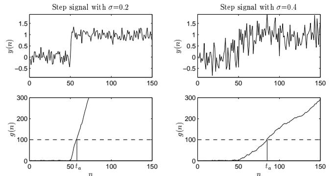
Fig. 2. Detection of a step change in a signal with a GLR detector, for two levels of additive Gaussian noise. The change point is at  $n = 50$ .
