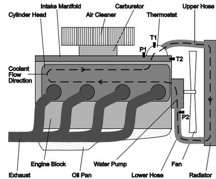
Fig. 4. Engine schematic with sensor placement (T1, T2, P1, P2).
