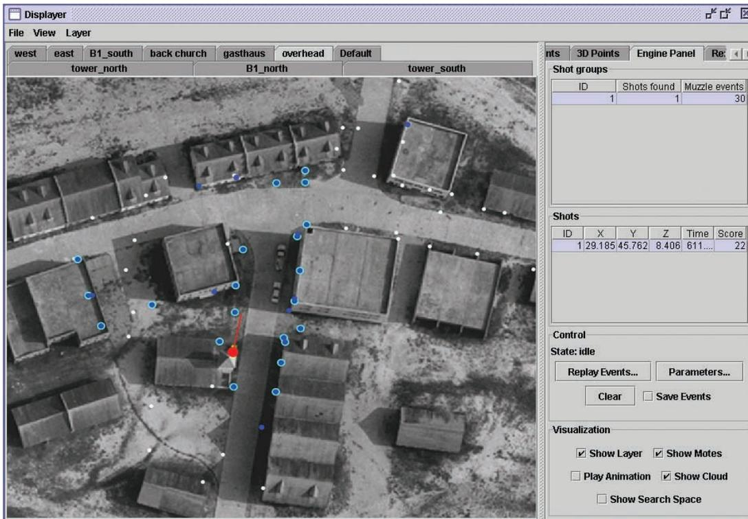
**Figure 2. PinPtr interface. In an overhead shot of the test area, the red dot shows the estimated shooter position, and the red line indicates the direction of the shot. The coordinates, including the elevation (8.4 m), are displayed on the right-hand side. Colored circles and dots show the sensor locations: white—no detection; blue—detection; cyan—line-of-sight detection.**
