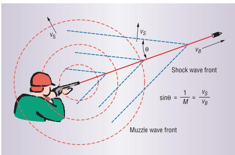
**Figure 1. Acoustic events generated by a shot. The muzzle blast produces a spherical wave front that travels at the speed of sound ( $v_s$ ) from the muzzle. The supersonic projectile generates a shock wave in every point of the trajectory, producing a cone-shaped wave front (assuming the speed of the projectile is constant  $v_B$ ). The projectile's Mach number  $M$  determines the angle of the shockwave cone.**
