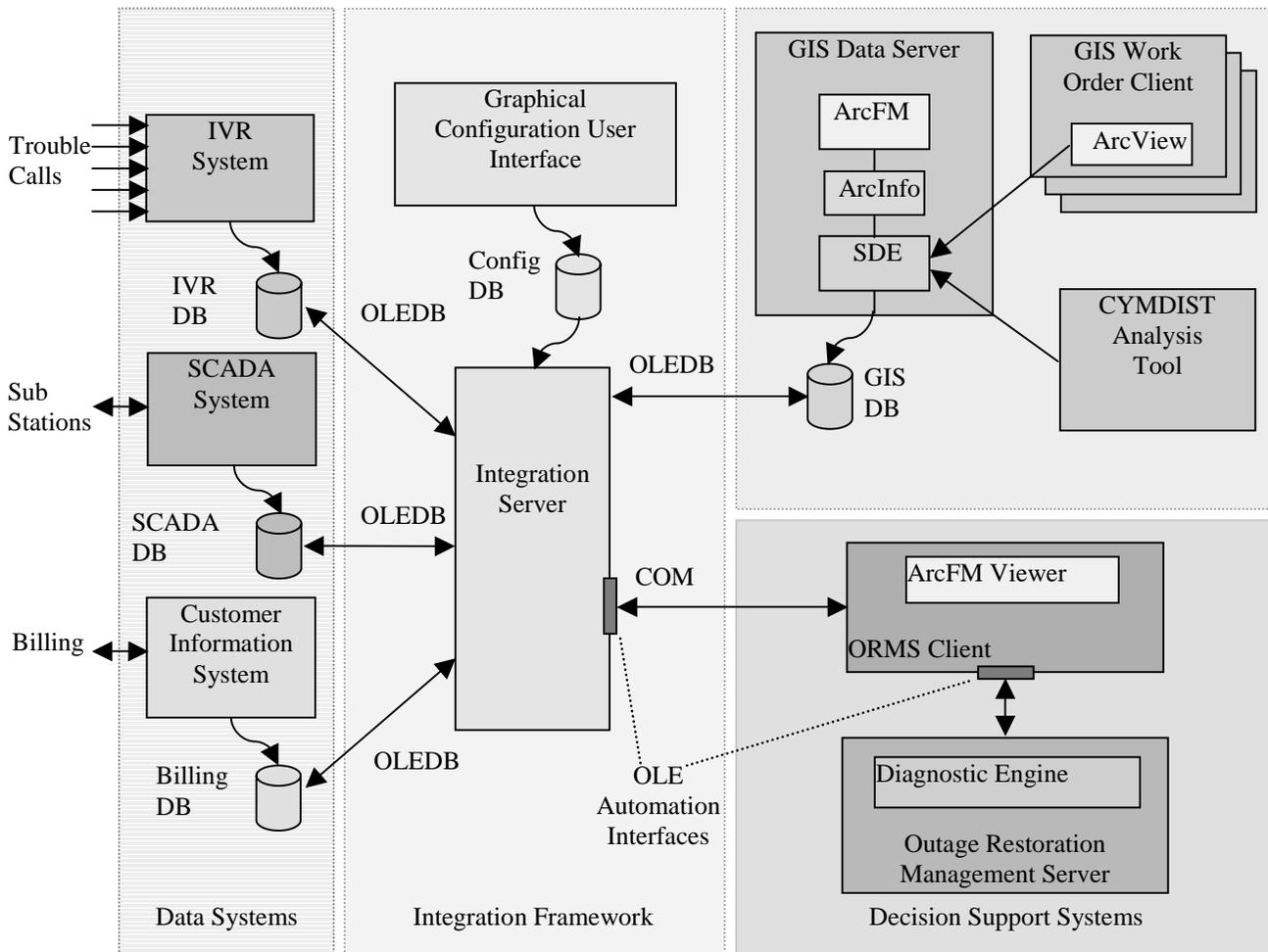
Fig. 1. The Integrated Distribution Management System Architecture
