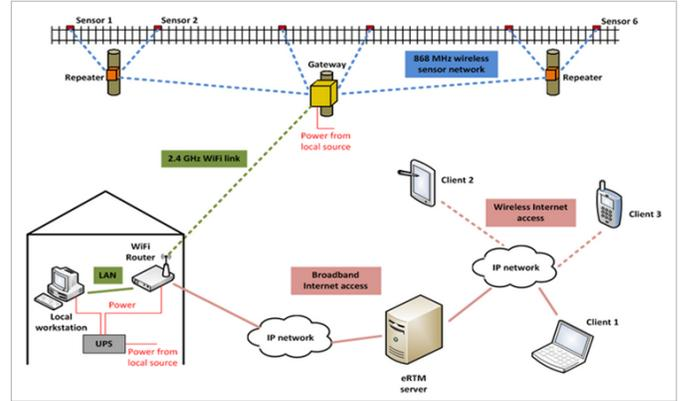
Figure 3. eRTM Generic System Architecture<sup>1</sup>
