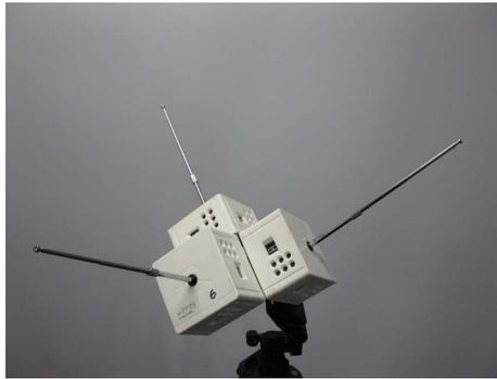
**Fig. 1.** Antenna array implementation using three XSM nodes.
