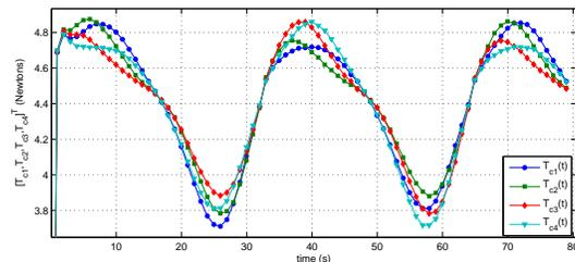
Fig. 11. Corresponding control thrust commands  $T_c$  for test flight.
