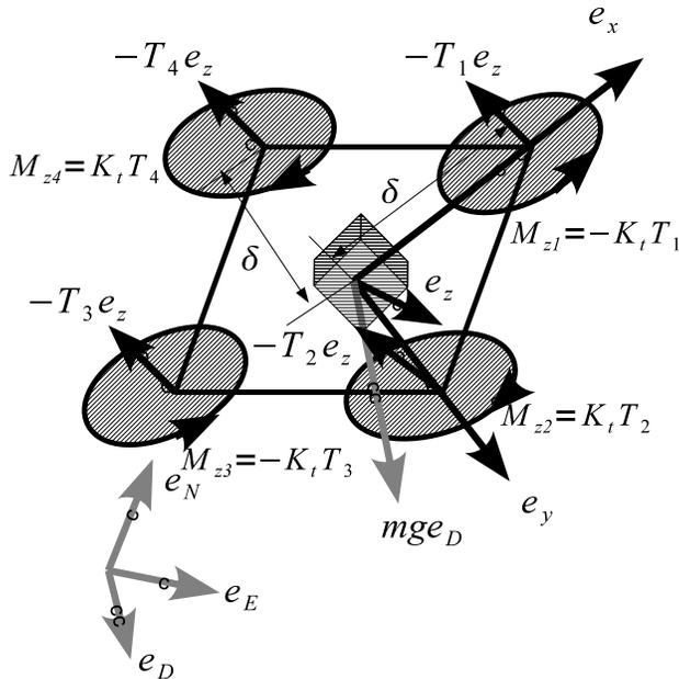
Fig. 3. UAV with depiction of inertial and body frames.
