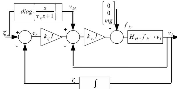
Fig. 6. Proposed inertial control system.
