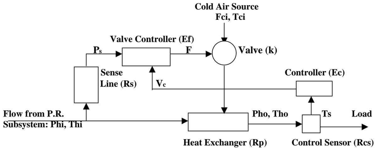
**Figure 3: The Pre-cooler Subsystem**
