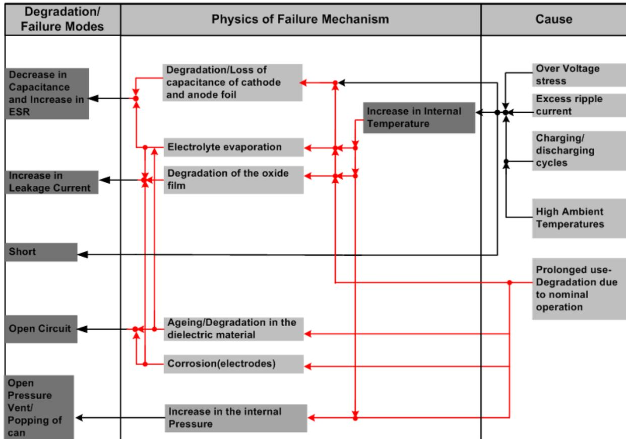
Figure 3: Causes, failure mechanisms and Failure modes in Aluminum Electrolytic Capacitor
