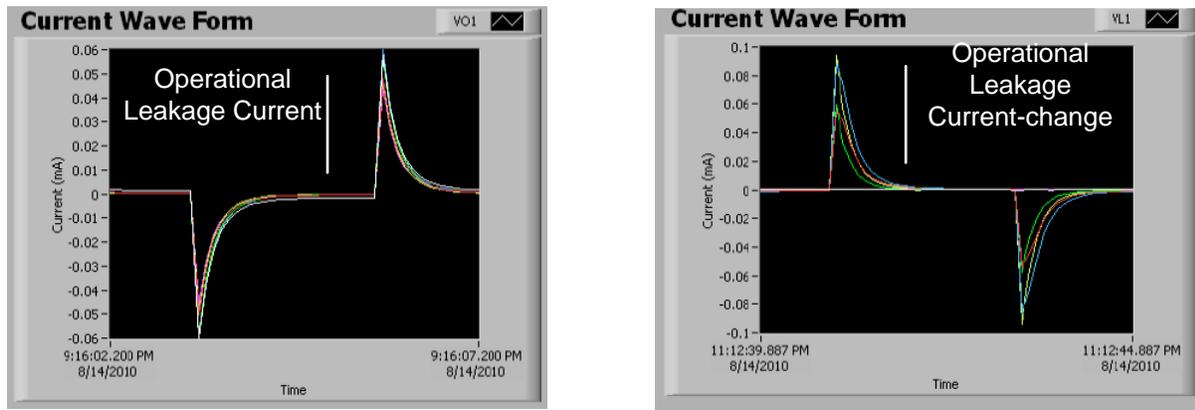
a) Leakage Current on Pristine devices
