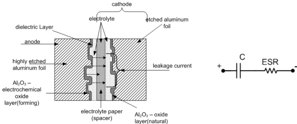
**Figure 4: Capacitor Structure and Equivalent circuit diagram**
