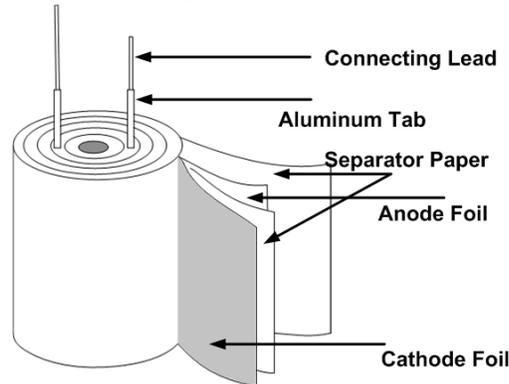
**Figure 2: Construction of Electrolytic Capacitor [1]**
