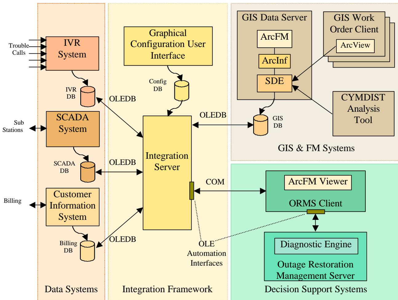
Fig. 1. The Integrated Distribution Management System
