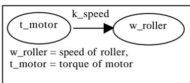
Fig. 5.1. TCG of motor and roller system
