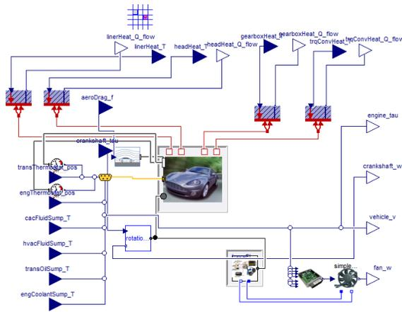
Figure 4: Driver vehicle model
