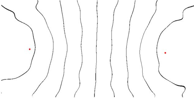
**Figure 2. Simulated map of zero expected received phase difference assuming nonideal RF propagation. The black hyperbolic curves represent the set of points where the expected phase difference is zero. The red dots are the transmitters' locations, positioned approximately 12ft apart. The wavelength is 2.45ft.**
