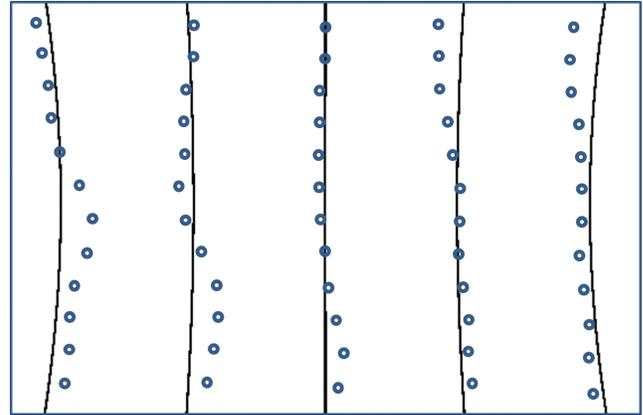
**Figure 3. Measured map of zero phase difference. The black hyperbolic curves represent the set of points where the expected phase difference is zero. The blue circles represent discrete positions where the phase difference was measured to be zero.**
