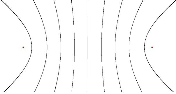
**Figure 1. Simulated map of zero expected received phase difference. The black hyperbolic curves represent the set of points where the expected phase difference is zero. The red dots are the transmitters' locations, positioned 12ft apart. The wavelength is 2.45ft.**
