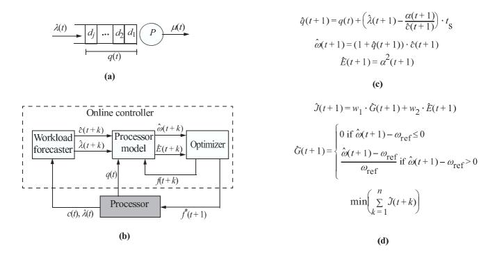
Figure 3: Application of online control to processor power management; (a) processor model, (b) overall structure of the online controller, (c) behavioral model of the processor, and (d) the cost function as a set-point specification
