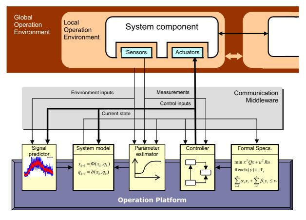
Figure 1: Key components of a self-managing computing system
