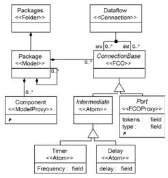
Figure 5 Package definition and dataflow
