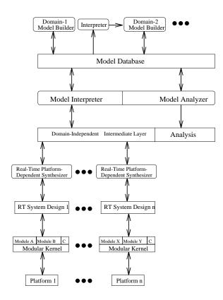
Figure 1: Model-Based Synthesis Architecture
