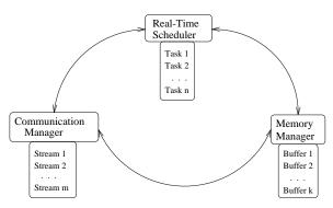
Figure 2: Basic Kernel Architecture
