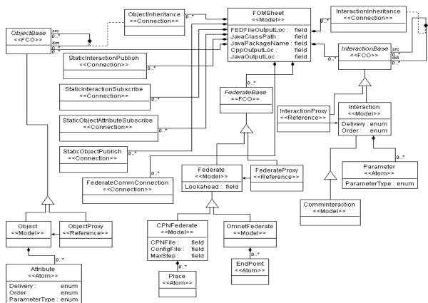
Fig. 1: Part of the C2 Wind Tunnel Meta Model
