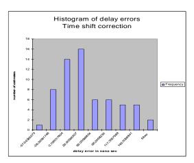
Figure 5 Histogram of errors in TDOA estimate when time-shift correction is used
