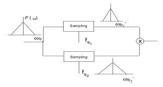
Figure 1 different sampling frequencies lead to frequency companding
