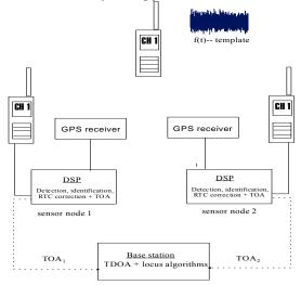
Figure 2. Schematic test setup. FRS radio transmits a pseudo random sequence containing the template. The two nodes find the template and send TOA estimates to the remote base station
