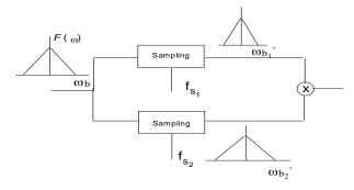
Figure 1 different sampling frequencies lead to frequency companding
