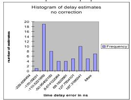
Figure 3 histogram of error in TDOA estimates without any correction applied
