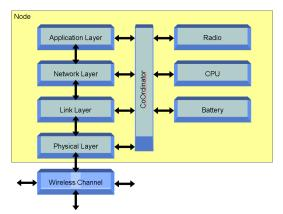
Figure 4. Code Structure for Each Wireless Node
