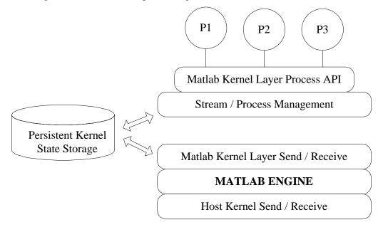
Figure 16. The Matlab kernel layer and interface to the host kernel
