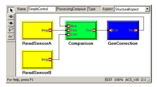
Figure 7. Compound SimpleControl, with a feedback connection from GenCorrection to Comparison
