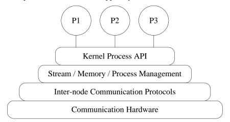
Figure 14. Organization of runtime kernel executing on a processor in the network
