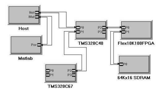
Figure 12. Resource Model showing the Matlab environment interfaced to the host
