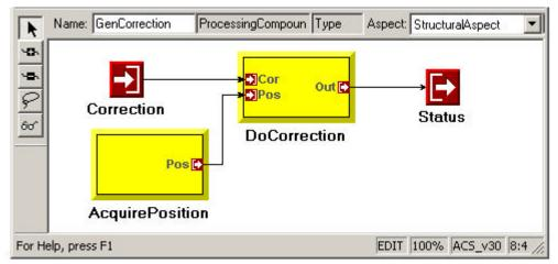
Figure 3. ProcessingCompound model GenCorrection, with submodels AcquirePosition and DoCorrection
