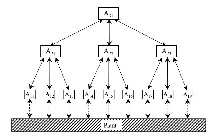
Figure 3 Schematic of vertical hierarchical control system.
