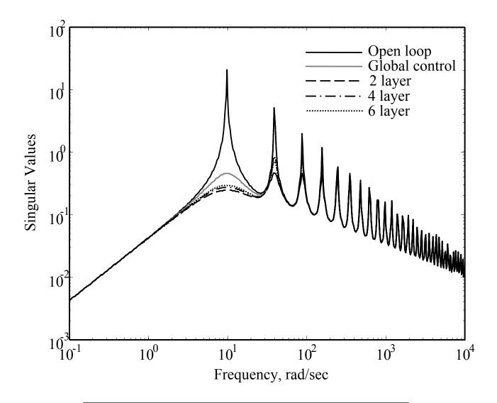
Figure 7 Comparison of closed loop performance between a centralized, global controller and several vertical hierarchic controllers.
