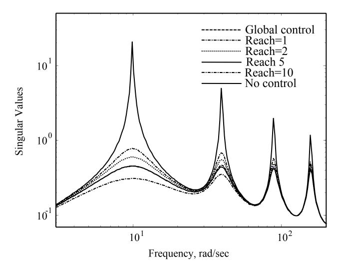
Figure 5 Zoomed view comparison of closed loop performance between a centralized, global controller and several horizontal hierarchic controlers of varying reach.
