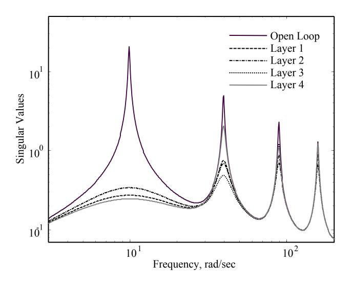
Figure 10 Zoomed view comparison performance for the 4-layer hierarchy when individual layers are designed with a cost weight 10 time larger than the other layers.
