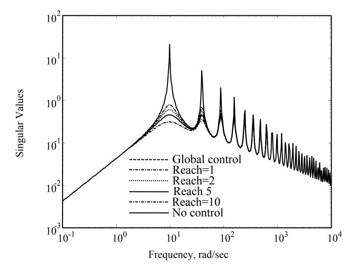
Figure 4 Comparison of closed loop performance between a centralized, global controller and several horizontal hierarchic controllers of varying reach.
