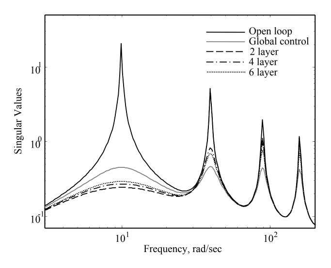
Figure 8 Zoomed view comparison of closed loop performance between a centralized, global controller and several vertical hierarchic controllers.
