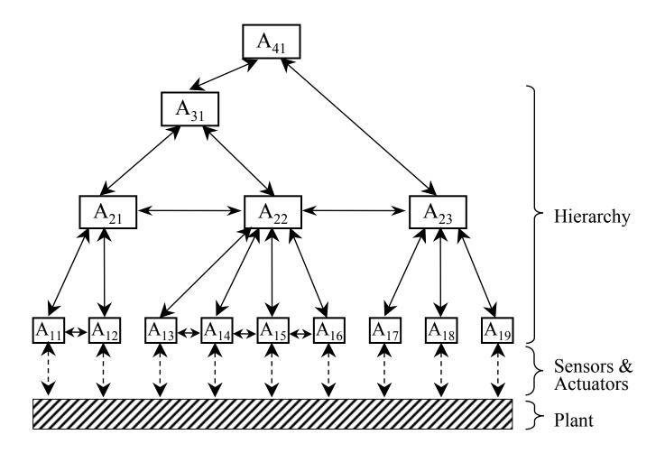
Figure 1 Schematic of hierarchical, decentralized control system.
