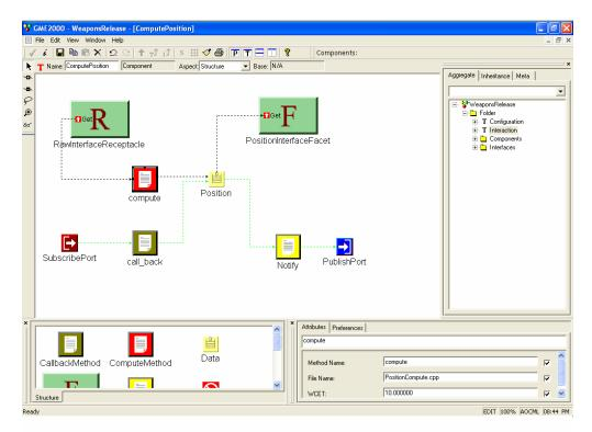
Figure 7: The Internals of the Compute Position Component
