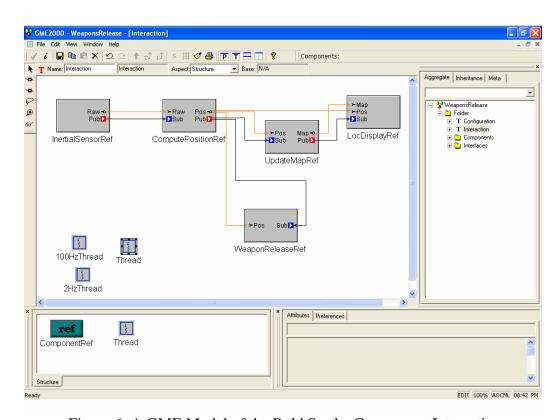
Figure 6: A GME Model of the Bold Stroke Component Interactions Figure 6 represents a simple model that contains five components. All
