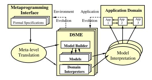
Figure 1: Process for Applying Model-Integrated Computing
