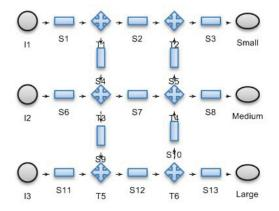
Figure 5. Domain-specific Model of Reconfigurable Conveyor Systems
