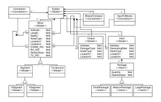
Figure 4. Meta-model of Reconfigurable Conveyor Systems
