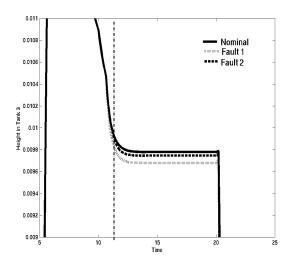
Figure 8: Experiment 2: Measurement is the height of liquid in tank 3
