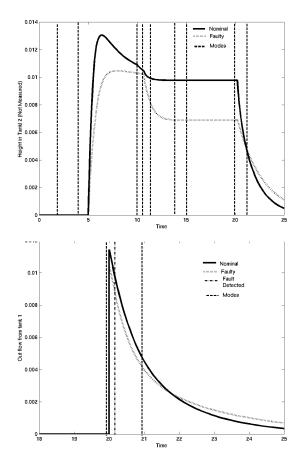
Figure 10: Experiment 4 -- Correct fault isolation occurs even though the observer predicts additional modes after the fault occurrence
