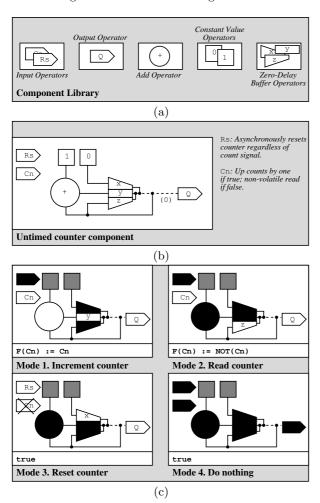
Figure 4: (a) A library of components (b) Components assembled into a counter (c) The modes that control the counter.
