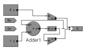
Figure 8: SMOLES/GME dataflow graph for the untimed aspect of the counter example.
