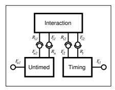
Figure 5: The Component-based architecture of TinyModes simulator
