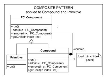
Figure 4: Composite pattern applied
