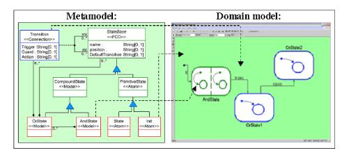
Fig. 1. Metamodel and model in MIC
