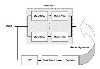
Figure 4: Adaptive Signal Analyzer
