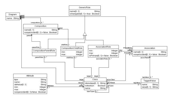
Figure 3 - The UML meta-meta model
