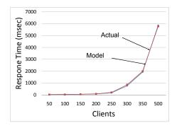
Figure 6: Response Time in Single Processor Machine
