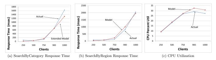
Figure 12: Model Validation for Configuration 2
