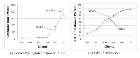
Figure 11: Model Validation for Configuration 1
