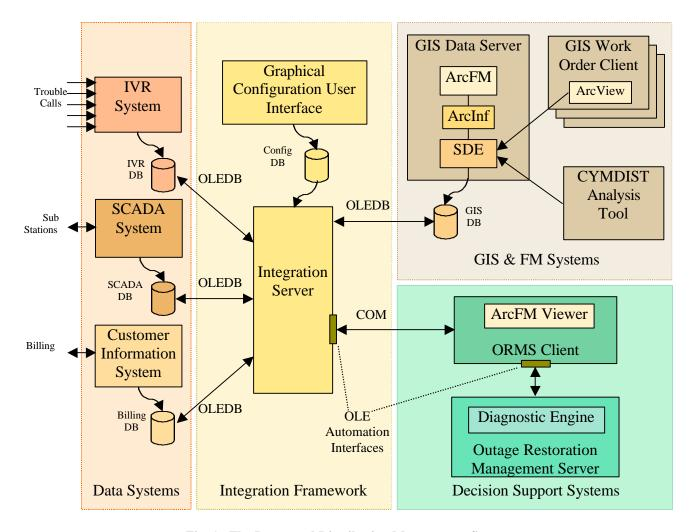
Fig. 1. The Integrated Distribution Management System
