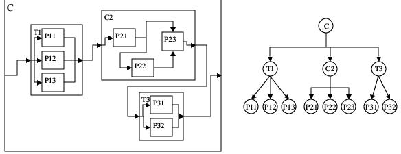
Figure 11: Hierarchical dataflow and its AND-OR-LEAF tree representation
