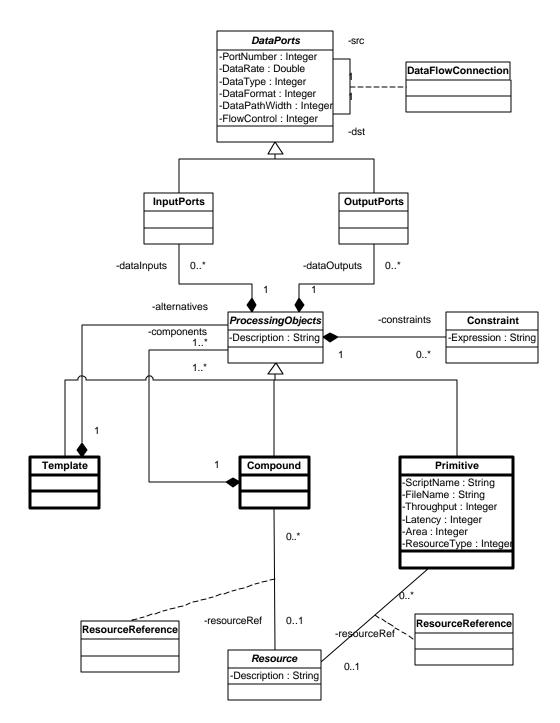
Figure 5: Metamodel of computational structure modeling
