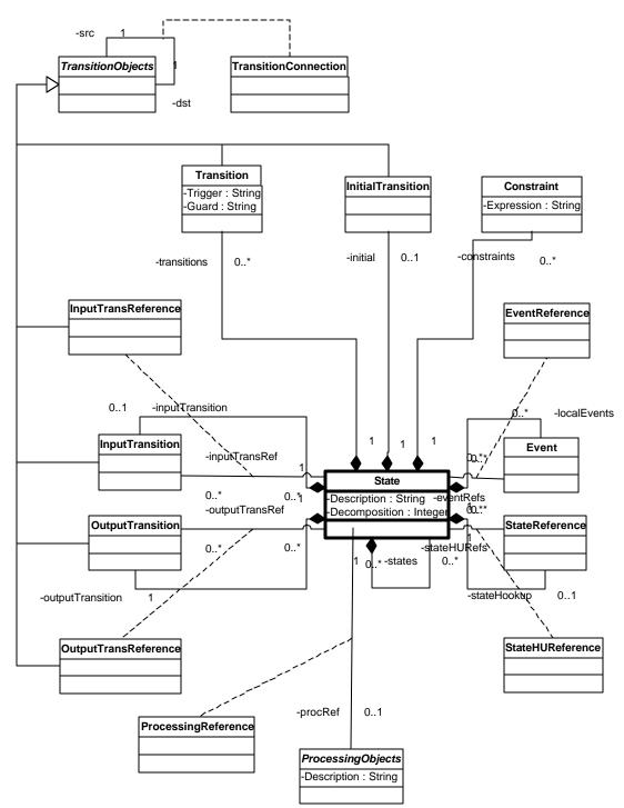
Figure 4: Metamodel of operational behavior modeling
