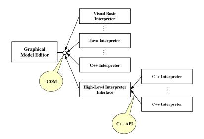
Figure 7: The GME Interpreter Interface Architecture
