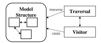
Fig. 5. Design of the ANEMIC translator includes automated visitor and traversal patterns for navigating the BON and collecting specialization information
