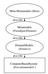
Fig. 1. The four layers of metamodeling
