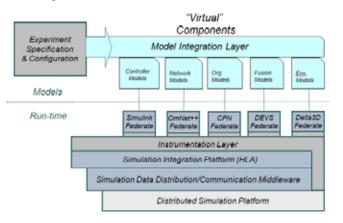
Figure 2: C2WT Simulation Architecture
