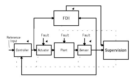
Figure 5 Fault Tolerant Control Architecture
