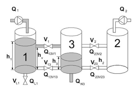
Figure 1 Three Tank System with Tank 2 Empty
