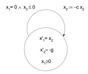
Figure 3 Hybrid Automaton of a Bouncing Ball
