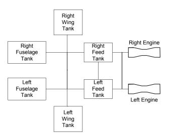
Figure 11. Simplified Aircraft Fuel System
