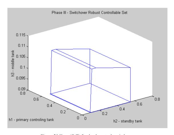
Figure 20  $K_{1,200}(\Omega,T)$  for the three-tank switchover
