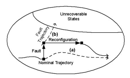
Figure 7 Single Step Reconfiguration
