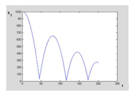
Figure 4 PWA approximation of bouncing ball
