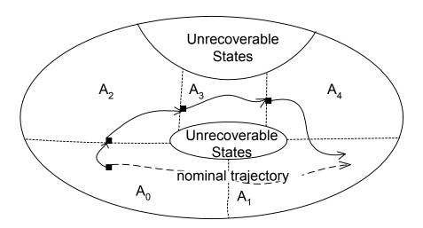
Figure 8. A multi-step reconfiguration process. Due to a fault the nominal trajectory cannot be followed. The supervisory controller dictates a multi-step process of guiding the system through regions  $A_2$ ,  $A_3$  and  $A_4$ , until the trajectory of the system returns to its regular course. At each step reconfiguration may be required.
