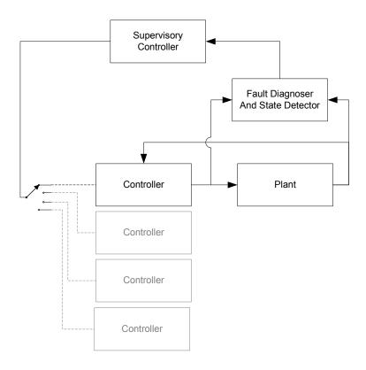
Figure 13. Architecture of the Aircraft Fuel Control System
