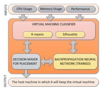
Figure 3. hALT architectural diagram
