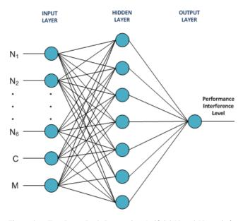
Figure 4. Two Layer Back Propagation Artificial Neural Network for Performance Interference Level Prediction
