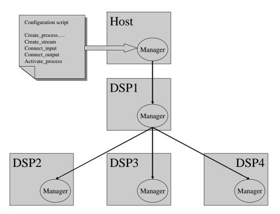
The reconfigurable hardware interfaces, and the flexible microkernel provide the facilities to implement system reconfiguration, however the problem of control and synchronization is critical. A global view of the system is necessary. Reconfiguration cannot be performed by the kernel alone.
