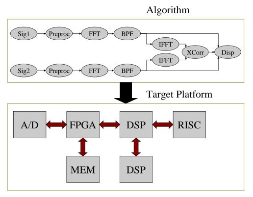
This figure represents the types of computations that execute on the target architectures. Algorithms are specified as a data flow diagram. These algorithms are mapped to heterogeneous architectures, containing a mix of implementation technologies that is optimized to the algorithm and its performance requirements.
