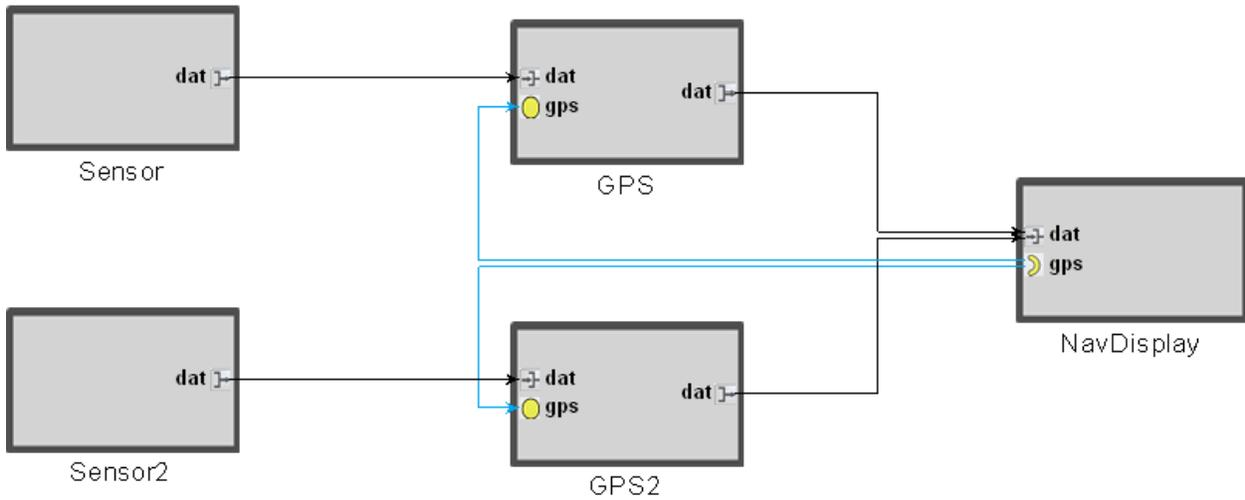
Fig. 2: GPS Software Assembly
