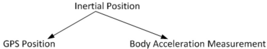
Fig. 4: Example of system functions for the GPS Assembly in Figure 2.
