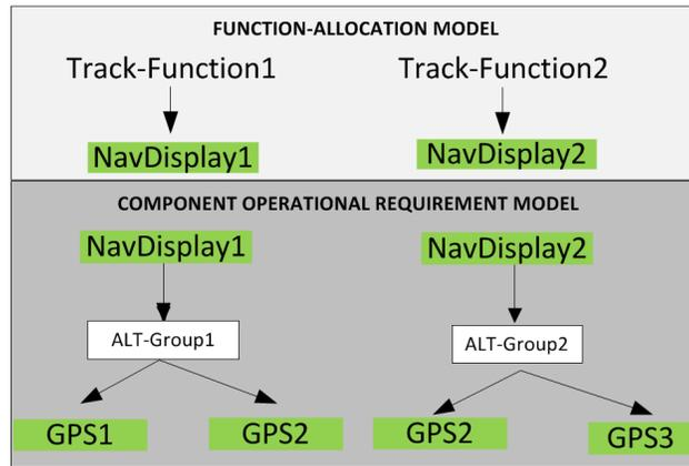
Fig. 13: Example 2: Equivalent Core Function Allocation Model and the Implicit Component Operational Requirements
