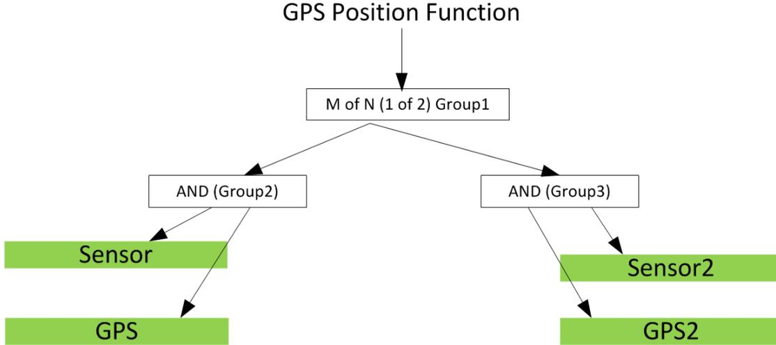
Fig. 5: Function allocation model for GPS-Position function in Figure 4
