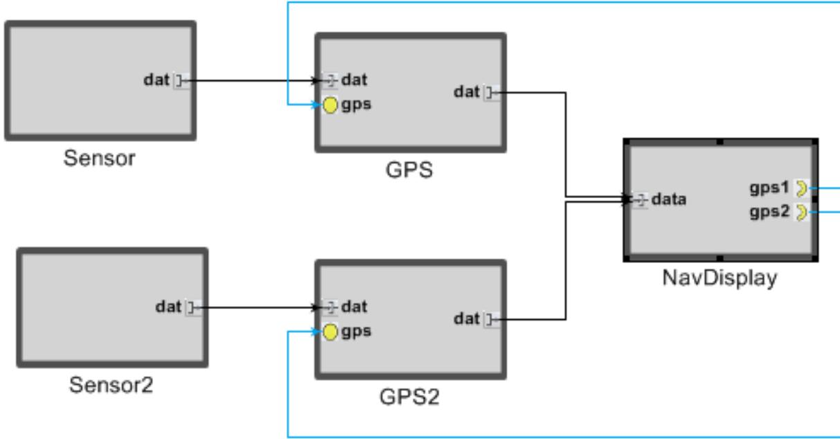
Fig. 6: Assembly model with modified NavDisplay.
