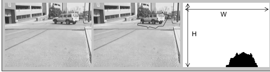
Fig. 7 Video detection. The frame on the left shows the input image, the frame in the middle shows the foreground and the frame on the right shows the video detection function.
