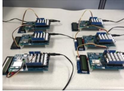
Fig. 8: The test bed comprising six Intel Edison compute modules, each mounted on an Arduino breakout board. Each board also has a Grove LCD screen attached to it.
