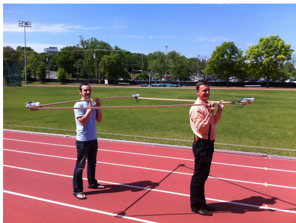
Figure 2: Experiment with three nodes exactly 9 feet apart moving around a running track, relative to an additional stationary node.
