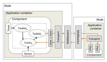
Fig. 1: Overview of the CHARIOT Component Model.
