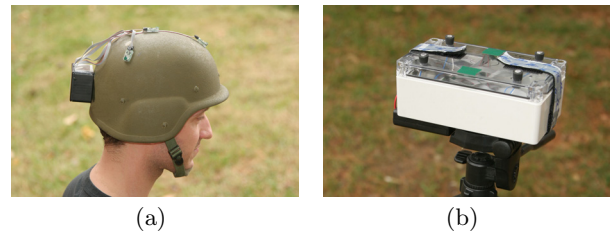
Figure 3: Sensor prototypes mounted on a kevlar helmet (a) and in a plastic box on a tripod (b).
